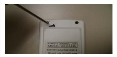
Remove all screws from behind the remote control and open.
