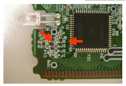
To make the conversion, remove the number 5 jumper from the remote's control board.
