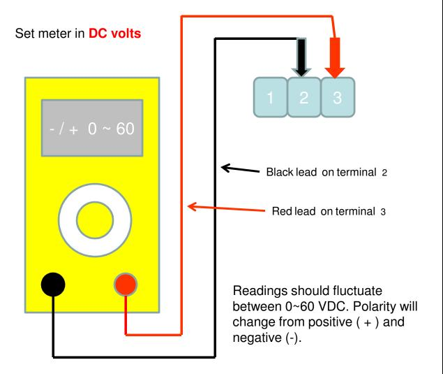
All positive readings would indicate a problem with outdoor unit and testing of the PCB will be required.
